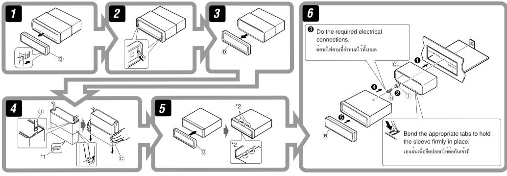
\*1 When you stand the unit, be careful not to damage the fuse on the rear.
